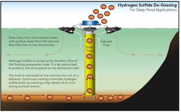
**Figure 2-** De-gassing a deep-water industrial pond by setting the intake all the way to the bottom. Deep dense water along with hydrogen sulfide is continuously drawn up to the surface of the pond where it will de-pressurize and vent into the atmosphere.
