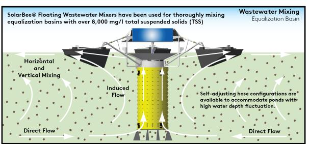
Figure 1- Set the intake near the bottom to keep solids suspended. Self-adjusting intake hose configurations are available to allow full mixing as the pond depth fluctuates.
