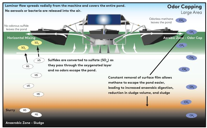
**Figure 3-** Odor cap an anaerobic pond by setting the machine to mix only the top 1-3 feet (0.5 - 1.0 m). This will effectively "cap" the anaerobic waters below with an oxygenated surface zone keeping odors at bay.
