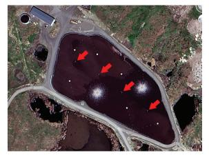
An aerial image shows location of the four new mixers as well as the eight aerators. After the mixers were installed to take over the mixing function, only two of the eight aerators operate at a time.
