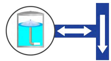
Separate: Water must move through the tank to continue down the line.
