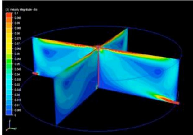
**Figure 2.** Computational Fluid Dynamics Modeling comparable to that shown in Figure 1 except that a SB1250PW is circulating the 2 MG of water. Continual mixing eliminates thermal stratification and prevents ice buildup.
