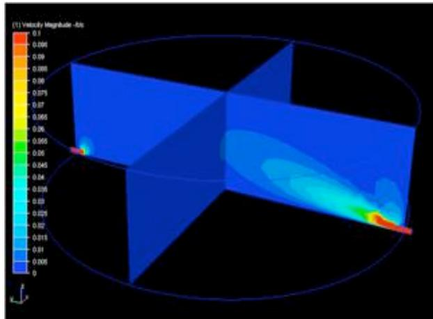
**Figure 1.** Computational Fluid Dynamics Modeling of a 2 MG tank with separate influent and effluent pipes indicates that most of the water is stagnant (blue) even during strong inflow (right, red) and moderate outflow (left, red).
