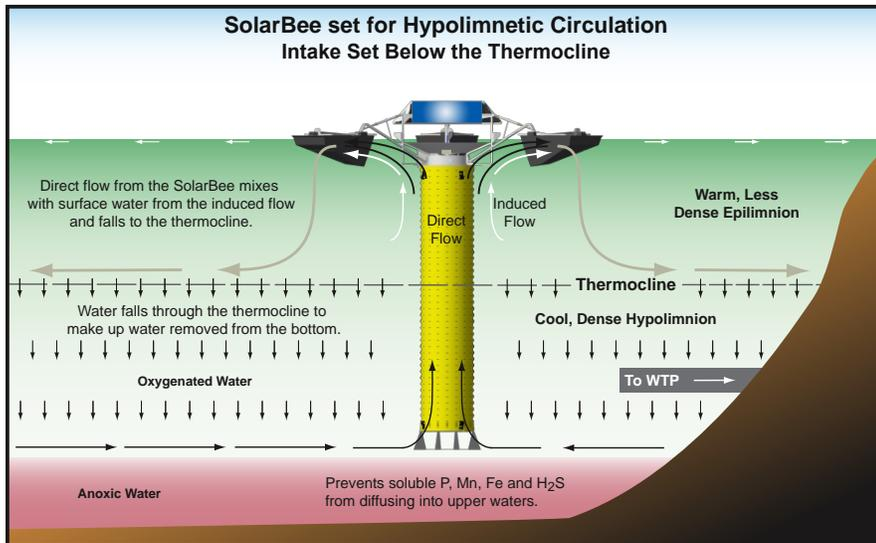
**Hypolimnetic Circulation-** The intake is set deep in the reservoir below the thermocline to continuously bring up and expose bottom waters to the oxygen-rich epilimnion and atmosphere.
